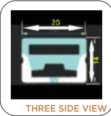
TSL-4559 Size : 20mmx14mm PCB:8mm,240LED MRP RS.: 775/-
