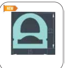
TSL-4565 Size : 10mmx15mm PCB:5mm MRP RS.: 650/-
